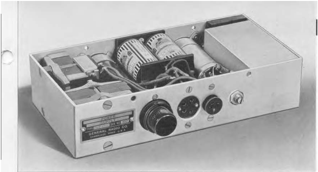
FIGURE 2. View of the power-supply unit showing the compact arrangement of parts.
